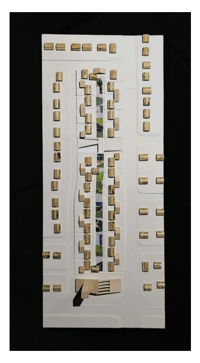
**◄** *site model. joined roofs and new topography collect water across the site. built to 1" = 30'-0" scale.*
